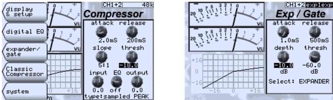
You can adjust the various parameters and use the "Select:" field to choose between "OFF", "EXPANDER" and "GATE". When either channel is actually expanding the status area will show "exp1" and/or "exp2" as shown here.
