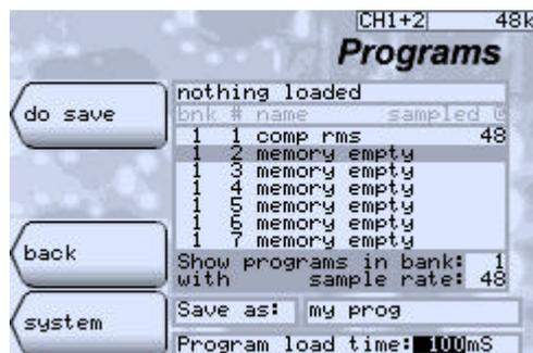
This picture shows the program save screen. The program load time can be set between 20mS and 9999mS (almost 10 seconds).
