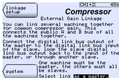
Here you can see that you can select the FX2000 external gain linkage to be off, or for the machine to a master or slave.
